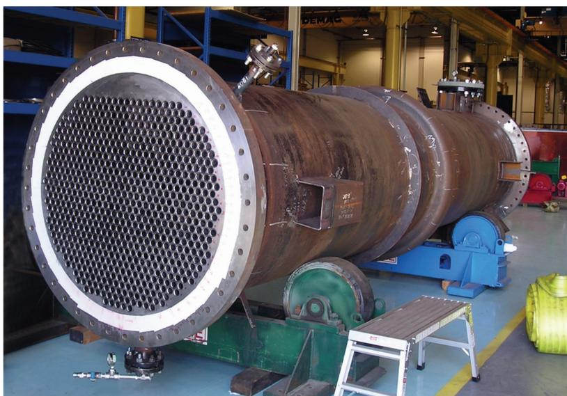
**Figure 3.** DDS exchanger during SS hydrotest.
