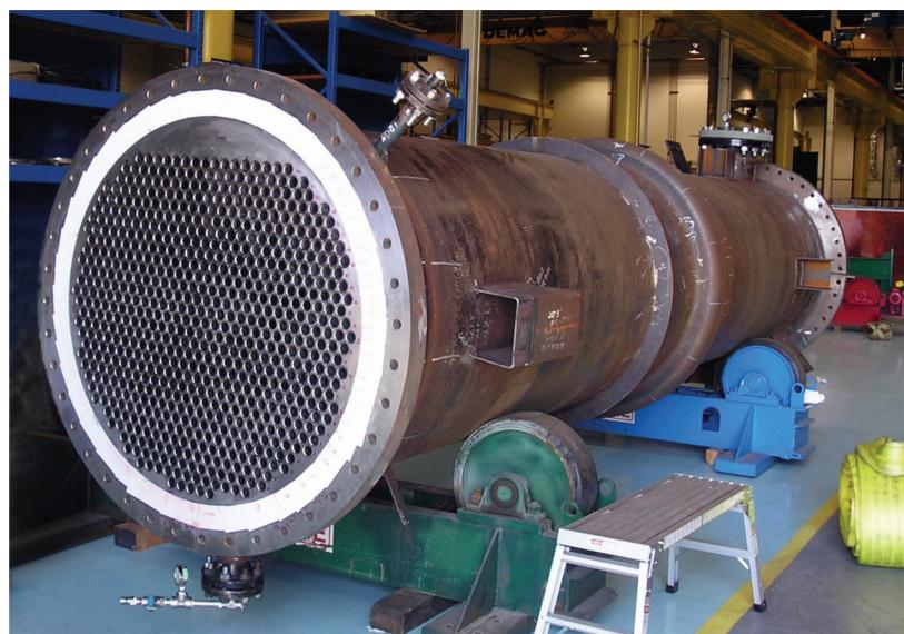
**Figure 3.** DDS exchanger during SS hydrotest.
